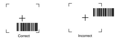
Figure 1-6 Imager Aiming Pattern: Bar Code Not Centered
